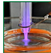
Figure 1: the micropulsed plasma jet during helium operation
