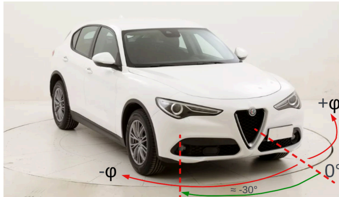
Figure 4.3: Azimuth \varphi definition for car pose estimation. In this image, an azimuth of \varphi = -30^\circ corresponds to the car slightly turned to present its right side (passenger side) towards the viewer. The right dashed line indicating 0^\circ represents the reference axis for this calculation.
