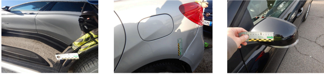
Figure 1.1: Illustrative examples of challenges in automatic damage assessment from photographs: confusing reflections and unrecognizable perspective on the left, shadows and unclear declared damages in the center, and presence of external objects like fingers and rulers on the right.
