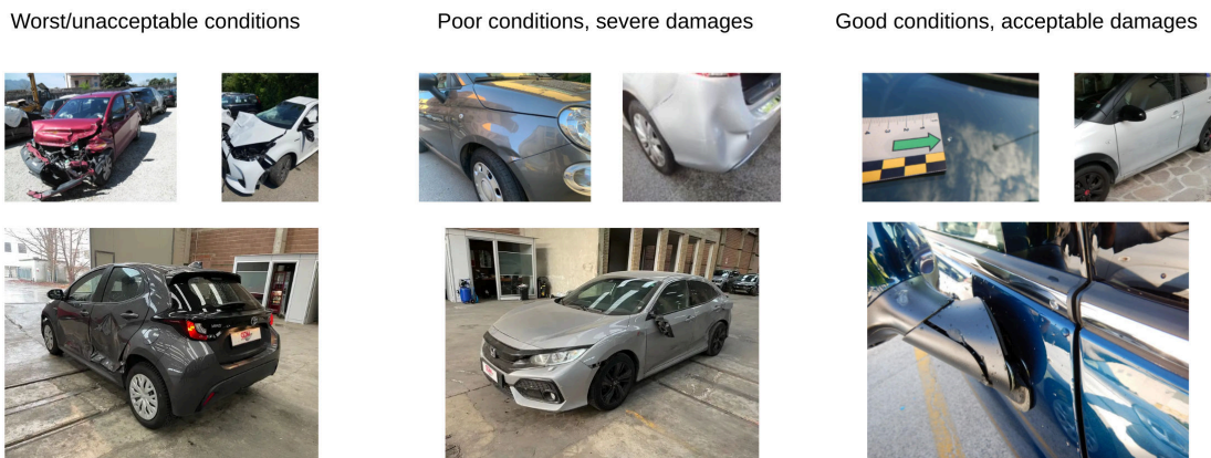
Figure 1.2: Examples showcasing the spectrum of damage severity: from non-repairable damages on the left to minor, sometimes even acceptable damages on the right.
