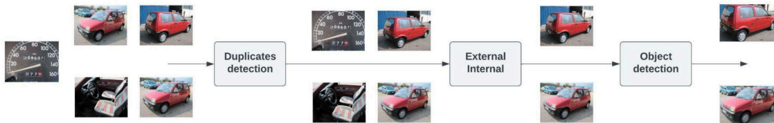
Figure 3.9: Flowchart depicting the sequential preprocessing steps for the dataset. Starting with near-duplicates removal, followed by an exterior image filter, and culminating with precise car localization to crop the vehicle’s area.
