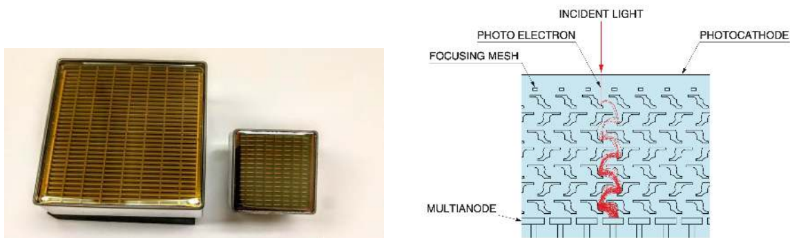
Figure 2.12: (Left) The MaPMTs selected for the upgraded RICH detectors with the 2-inch model (on the left) and the 1-inch model (on the right). (Right) Scheme of the internal structure of the MaPMT. From [83, 97].
