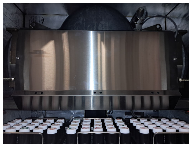
(b) Photo of the Quantulus 1220 detector schematically represented in Fig. 2. The movable sledges housing the 20 ml vials are also visible below. On the right and left sides of the metallic plate it is possible to see the lead shielding containing the coincidence PMTs.
