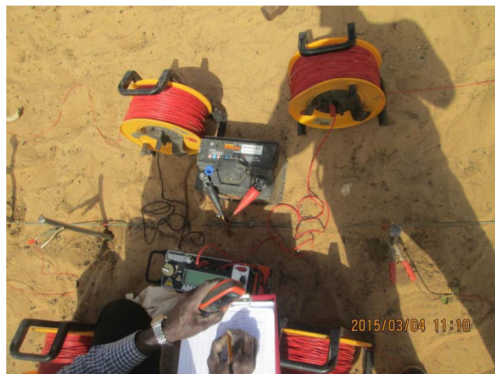
Figure 43 Resistivimeter used in VES survey
