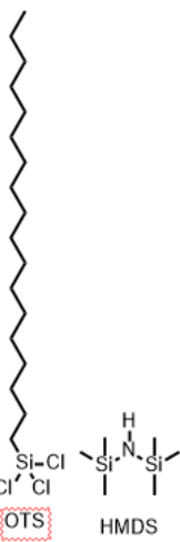
Figure 46: chemical structures of OTS and HMDS.
