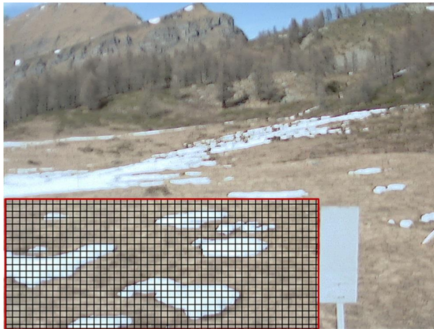
Figure 6.2. The region of interest (ROI) in red was chosen in the foreground to avoid problems related to distance, weather and excessive pixel size differences. The ROI was then divided using a grid with a grid cell size of 10x10 pixels. Nineteen rows and forty-nine columns result from the division.
