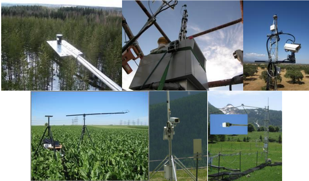
Figure 2.1 Some examples of the use of sensors in the field. (a) Skye sensor at Hyytiälä forest site (FI-Hyy, Finland), (b) S-fluor box at Duke forest (Durham, NC, USA), (c) AMSPECsystem at the Majadas del Tiétar site (Spain), (d) Ocean Optics sensor at Zeilaushen (Germany), (e) RGB camera at Torgnon site (Italy), (f) Cropscan sensor at Monte Bondone grassland site (Italy)
