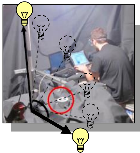
Figure 4.1 Set up used for the laboratory characterization. In the horizontal plane the cosine receptor is fixed (in the picture the FSF IS, rounded in red). The rotating arm allows a movement from the vertical position up to the horizontal one. The arm stops each 5.625 degree. The receptor response at 17 zenith angles has been characterized per each sensor.
