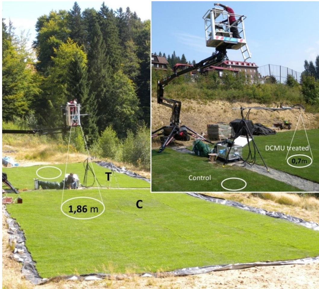
Figure 7.1. Experimental setup at Bíly Kriz site. The two lawn carpets are depicted in Figure. C is for control and T is for herbicide treated carpet. The position of the portable spectrometric system hosting two Ocean Optics spectrometers and the ASD spectroradiometer is shown together with the dimension of the field of view of each instrument.
