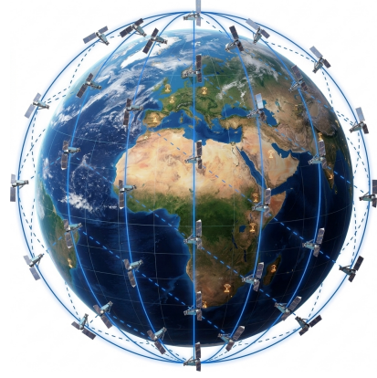
Fig. 1: The Iridium NEXT constellation: 66 satellites in 6 polar orbital planes forming a continuous spatial mesh [15].
