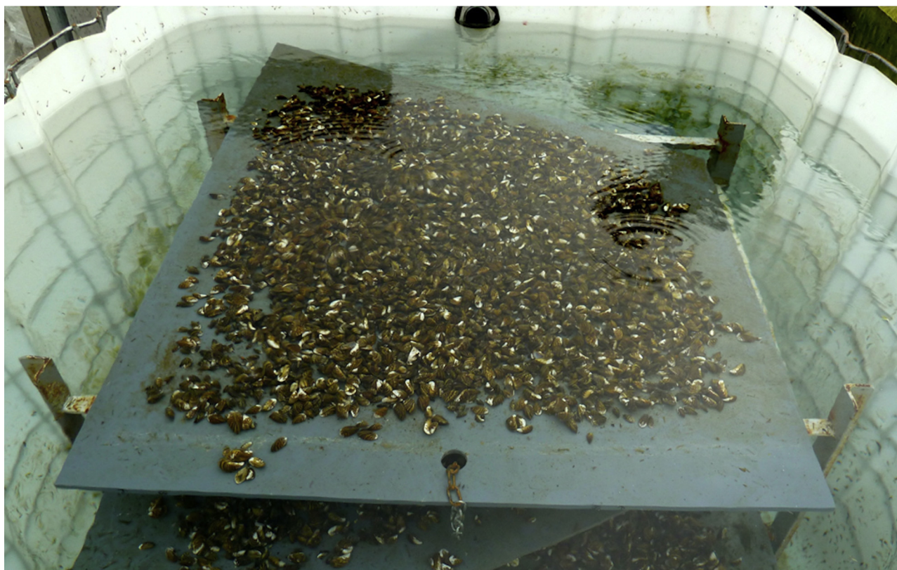
Fig. 3. Plexiglas® panels with bivalves placed horizontally inside the attachment tanks.
