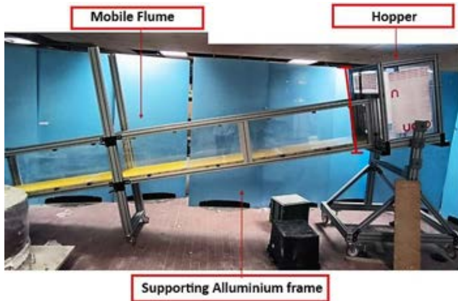
Fig. 5.6: Experimental setup - University of Milano-Bicocca
