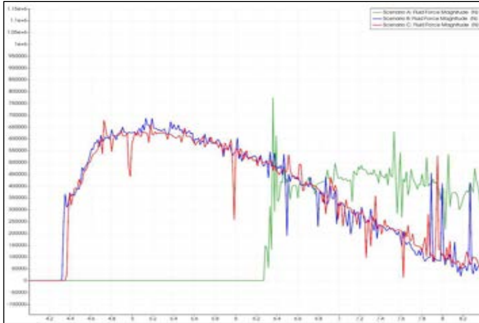
Fig. 4.33: Comparison of impact force trends, Scenario A-Scenario B–Scenario C
