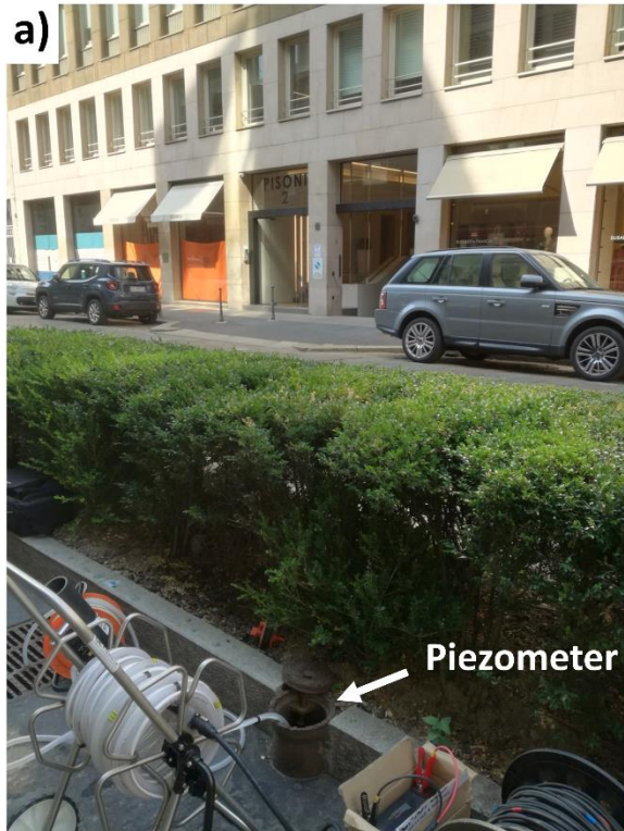
Figure 3.2 – (a) Example of groundwater temperature monitoring in urban areas: (b) temperature-depth profiles by manual vertical logging and (c) automatic recording of temperature time-series.
