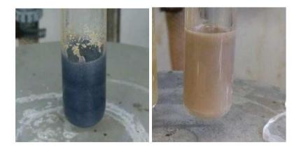
**Figure 80.** Picture of the micellar reaction of BTBT-Br with phenylboronic acid in a surfactant dispersion of PiNap-750M (left) and K-EL (right). The blue colour of the reaction performed in PiNap-750M is peculiar, and only seen after the addition of the catalyst and the NEt<sub>3</sub> to the surfactant dispersion.
