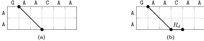
Figure 3.2: (3.2a) diagonal j = 1 : lce_{S,P}(0, 1) = 2 , thus the 0-FRP reaches the last row of the table and k_E -EXT correctly returns pair (2, 0) . (3.2b) diagonal j + d = 2 : R_d(|S|, |P|, ST_{P,S}^*, 1, 2) returns (r_d, c_d) = (1, 3) (as lce_{S,P}(2, 4) = 0 ): since r_d = |S| - 1 , this path reaches the last row of the DP table, and k_E -EXT correctly returns pair (3, 1) .
