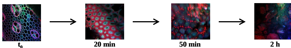
Figure 2 (44). Fluorescence images of a stem of switchgrass treated with ionic liquid ([emim]Ac). Left to right: the section before treatment, 20 minutes after treatment, 50 minutes after treatment, and two hours after treatment. The organized plant cell wall structure has been completely broken down.
