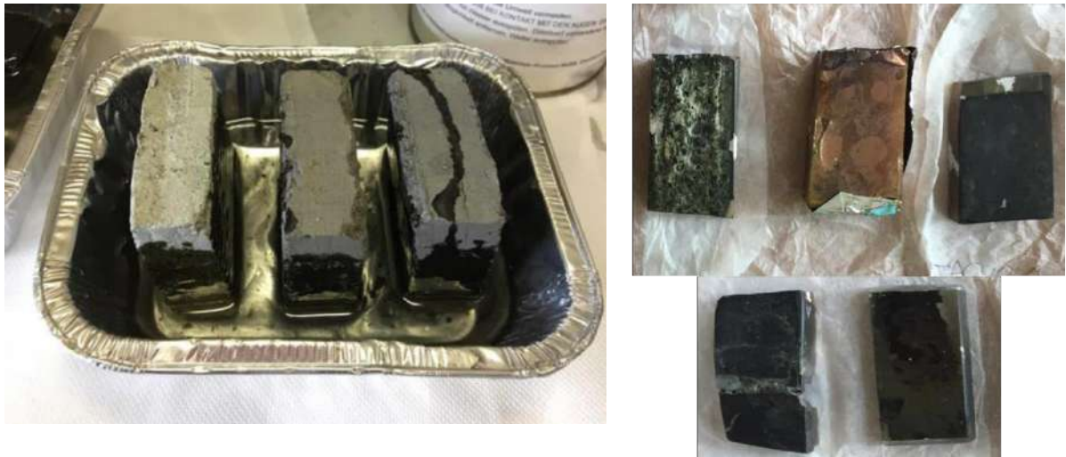
Figure 107 – epoxic resin embedding process (left-hand side); finale result on polished sections (right-hand side)
