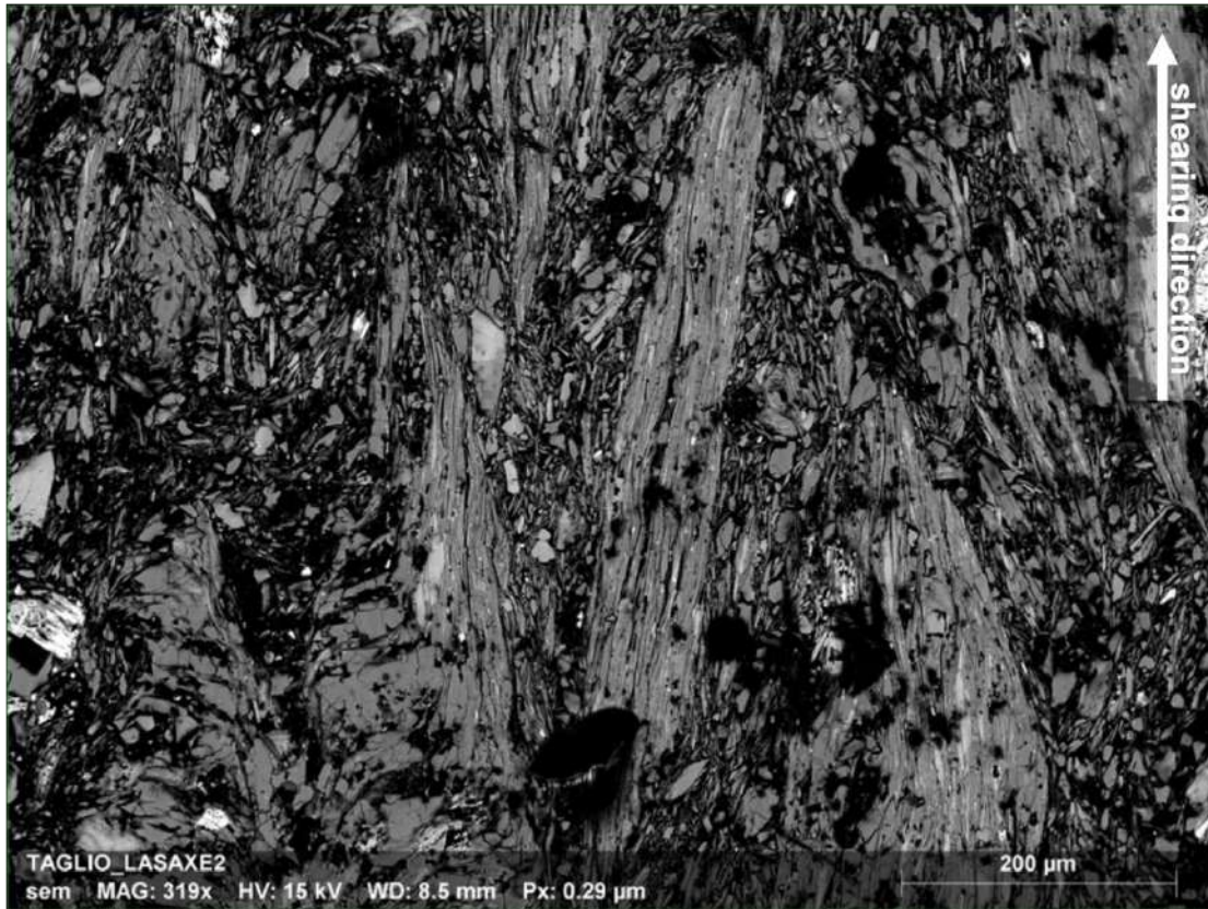
Figure 116 - SEM of DPRI test sample, with a preferred alignment of phyllosilicates and a presence of graphite (gr; black spots)
