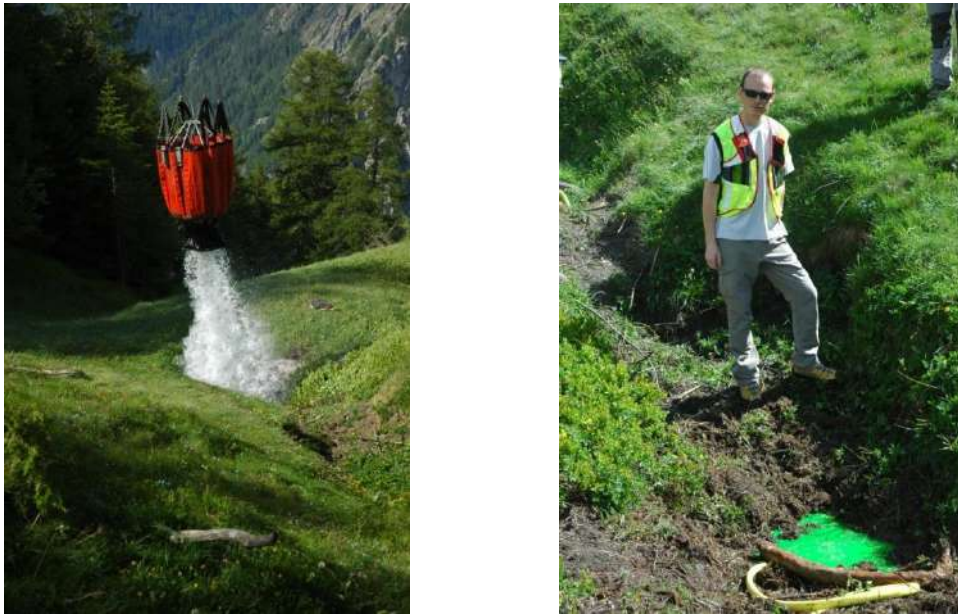
Figure 71 – (on left) saturation of the trench before starting the tracer test; (on right) close up on injection point
