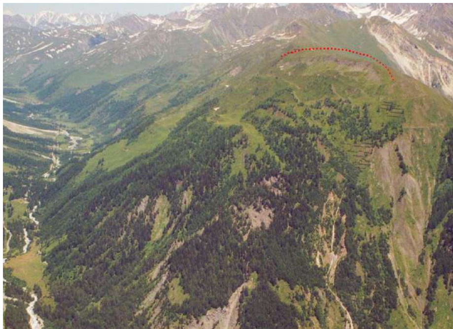
Figure 34 - The left-hand flank of the Ferret valley. The photo is taken from the Mont Chetif and shows the deep-seated gravitational slope deformation and the Mont de La Saxe rockslide. Dotted line represents the main scarp.
