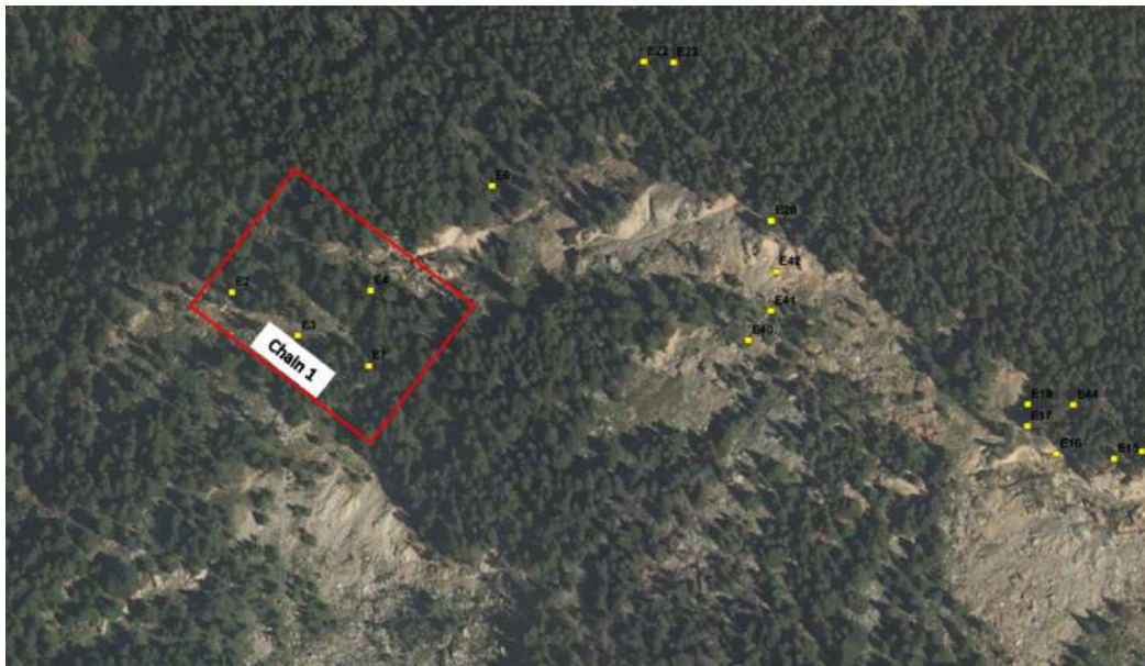
Figure 192 – distribution of extensometers along the lower scarp of Ruinon rockslide (Chain 1)
