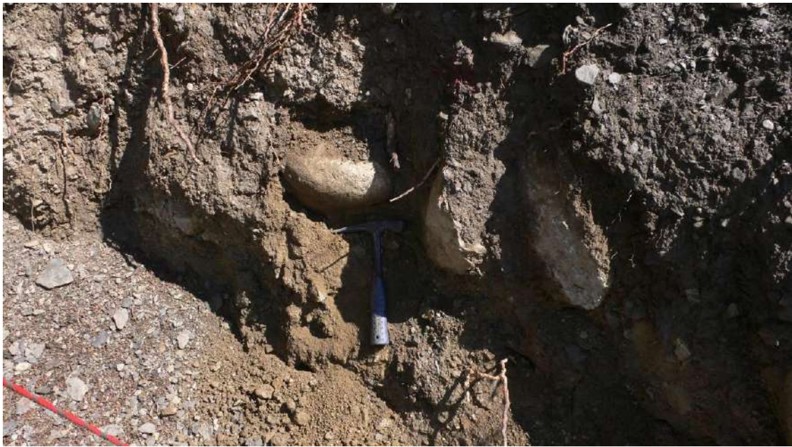
Figure 41 - Glacial till and its colluvial products present in the lower portion of the central sector of the rockslide
