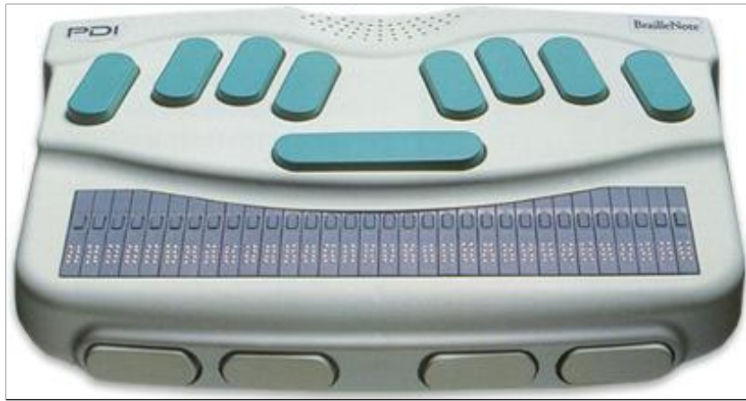
Figure 3.2: A Braille keyboard with chording keys
