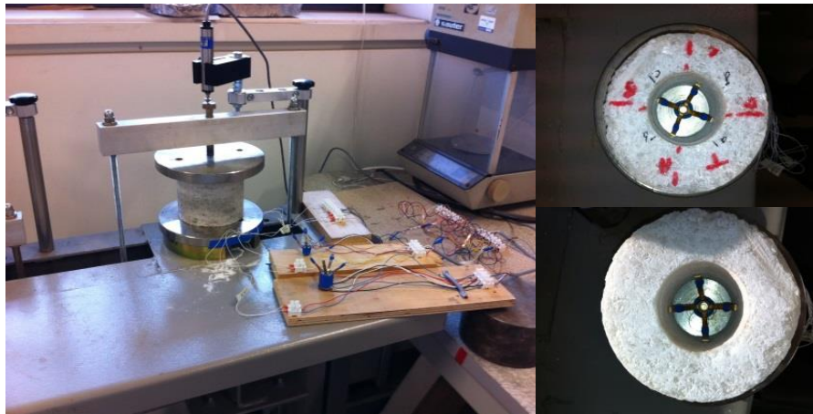
Figure 5-9 measuring device inside TWHC specimen
