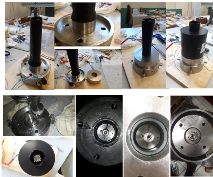
Figure 5-16 assembled inner membrane into lower part of apparatus (upper side), installation expandable sealing piece into inner membrane for upper part (lower side)
