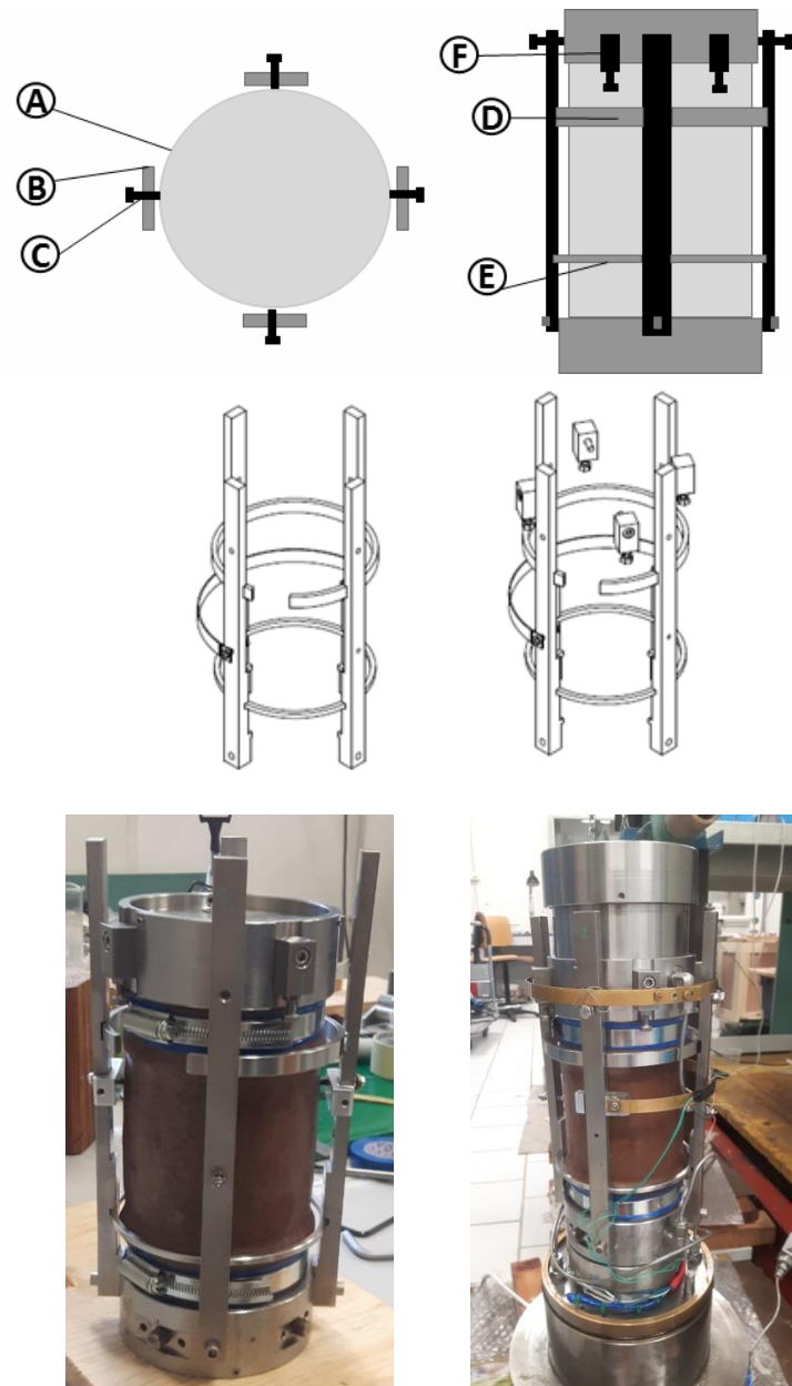
Figure 5-14 centering, safety system,
