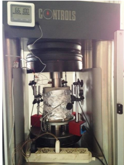
Figure 4-46 tri-axial cell equipment's with temperature bands, and thermocouples
