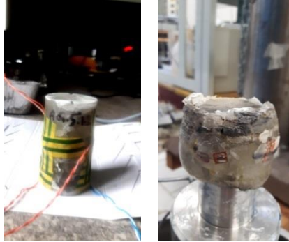
Figure 4-99 rock salt specimen before and after creep test (55C).
