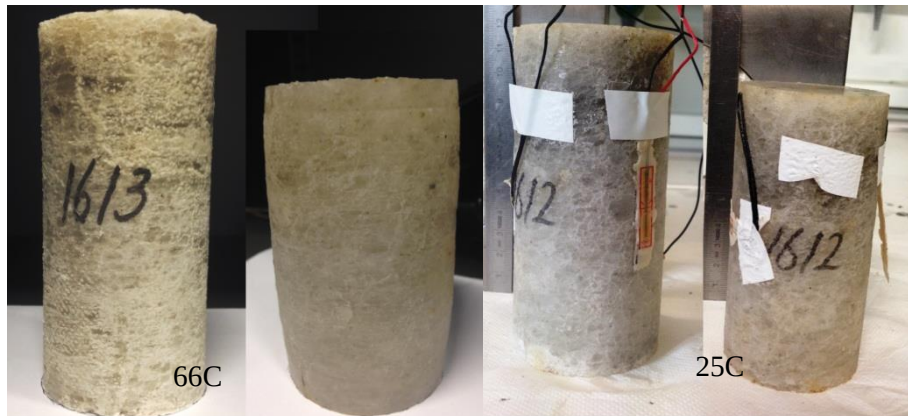
Figure 4-77 two specimens before and after creep tests with different temperatures.
