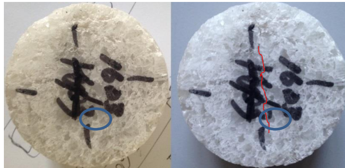
Figure 4-14 ) tensile crack easy along grain boundary rather than through grain (Italian salt photo before and after Brazilian test)
