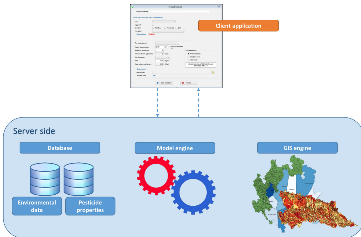
Fig. 3. Component diagram of the software system — There is a client application, which communicates with a server tier realised by a database, a model engine and a GIS engine.
