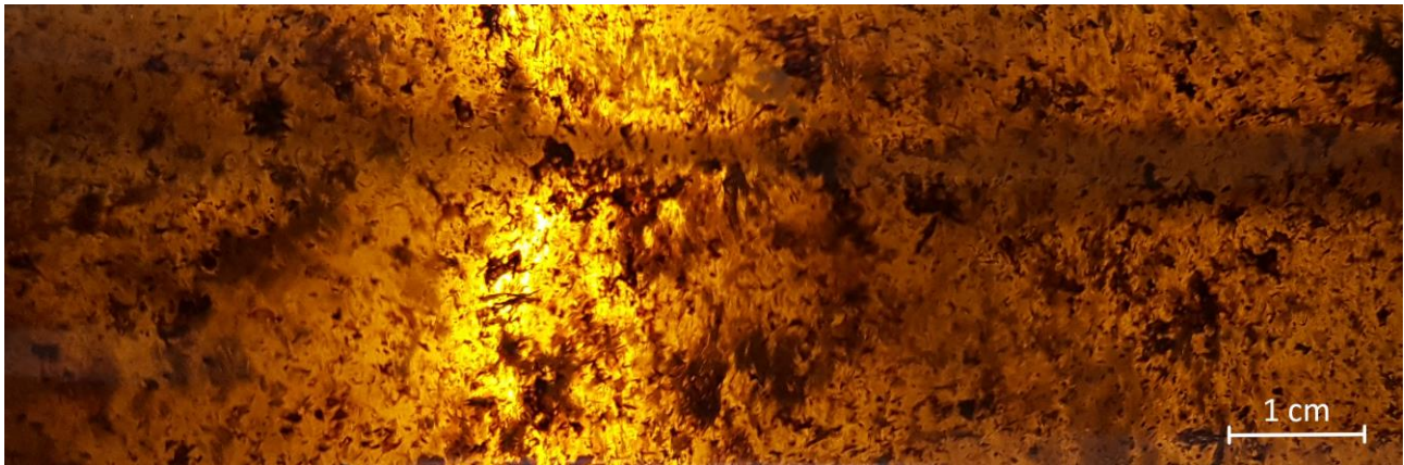
Figure 107 – Picture of a vial positioned in front of a light source containing a dispersion of TC1 modified lignin in a 0.5 M NaOH solution. The image was recorded with a digital camera.
