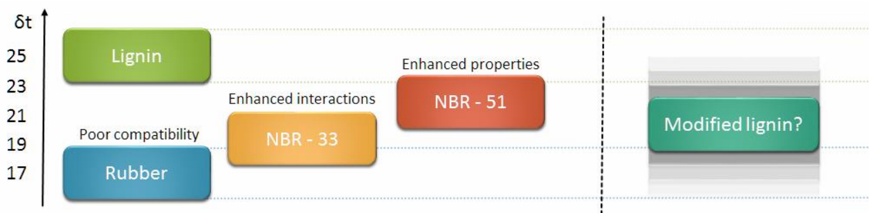
Figure 114 – Differences between cohesive energy density or solubility parameter ( \delta t ) for lignin and different rubbers.
