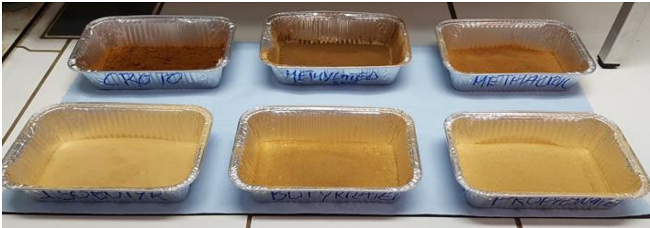
Figure 117 – Modified lignins after drying. From top left to bottom right: crotonated, methylated, methacrylated, isobutyrate, butyrate and propionate.
