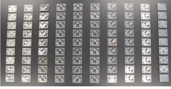
Figure 4. Al-alloy OMT plates manufactured through wire EDM.
