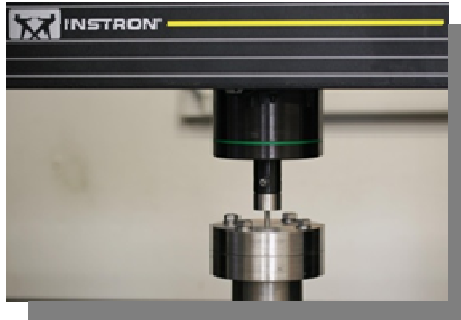
Figure 2.21. Experimental setup used to perform small punch tests.
