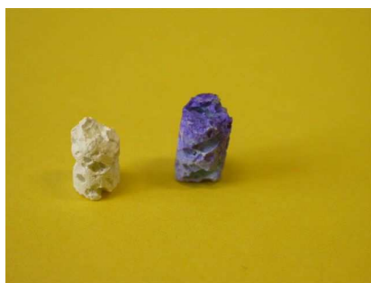
Figure 2.1 Thionine acetate colorimetric assays on untreated HA (left) and plasma polymerised AAc-HA (right).
